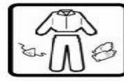
Cover exposed skin. When working in unventilated area wear disposable face mask
